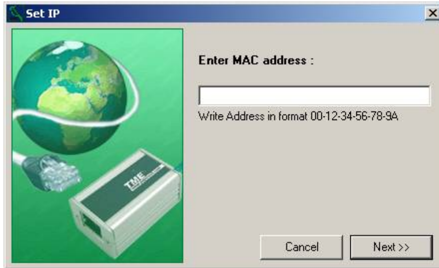
Fig. 13 – changing the IP address of a thermometer with a known MAC address
