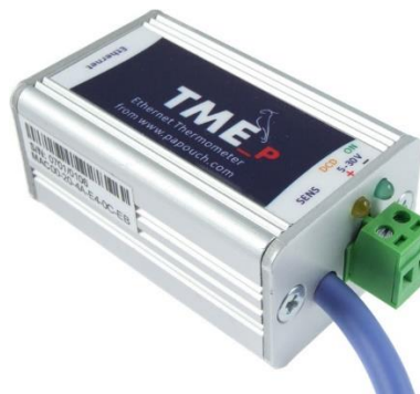
Fig. 5 – Variant TME_P (with 7 - 30 V power supply)
