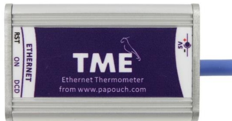
Fig. 4 – TME version (with 5 V power supply)
