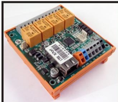
Board with a DIN rail
