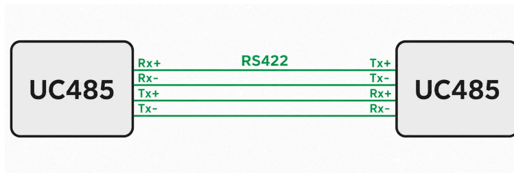
Fig. 6: RS422 connection example; both modules have termination connected
