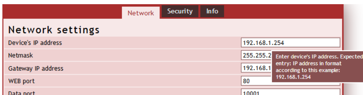
fig. 3 – pop-up help shown when the cursor hovers over an item – screenshot from a different device
