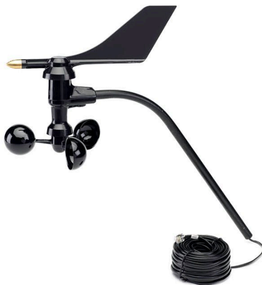
Fig. 15 – wind speed and direction sensor
