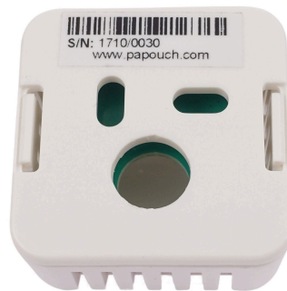
Fig. 14 – bottom side of the CO 2 concentration sensor
