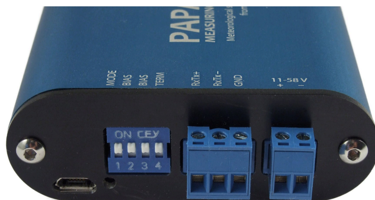
Fig. 3 – panel with RS485, power and configuration USB connectors
