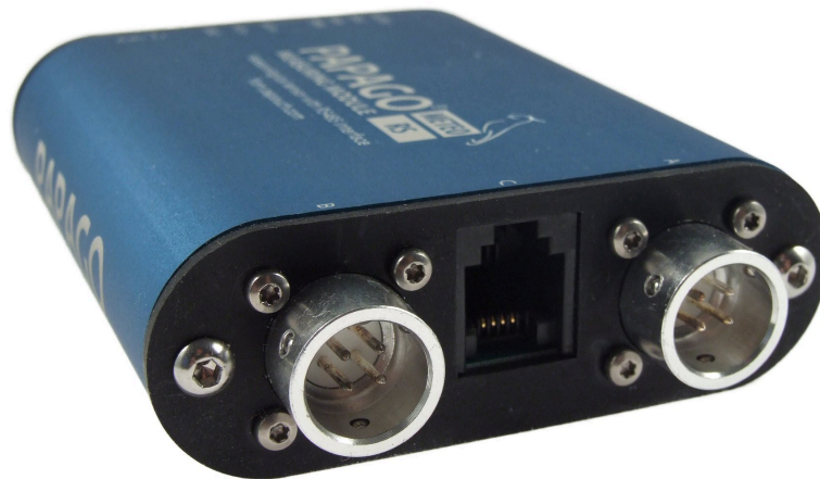
Fig. 2 – front panel with sensor connectors
