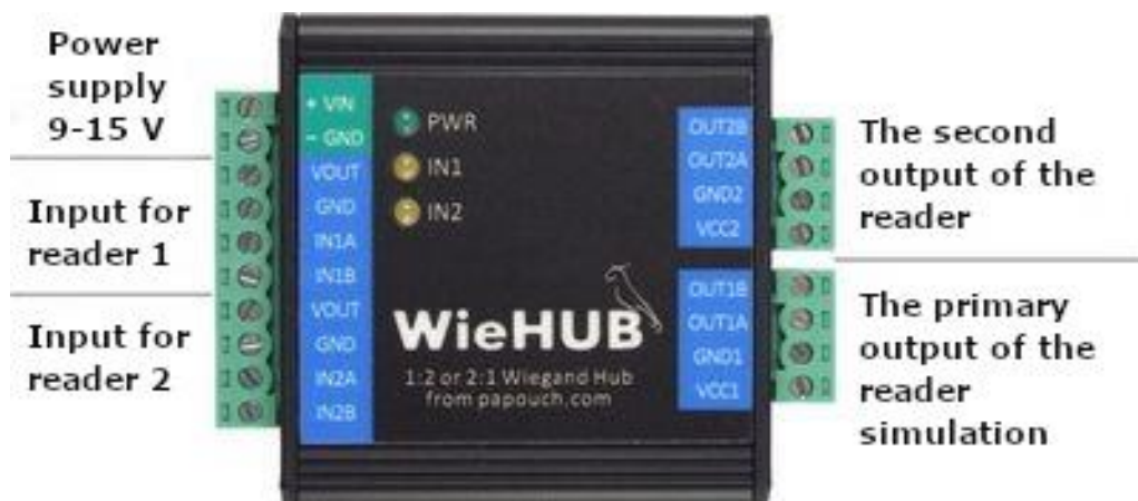
Fig. 4 - Terminal block on the transmitter
