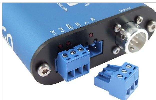
fig. 19 - status indicators above the digital inputs and outputs
