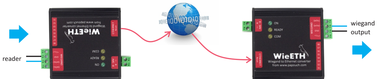
Ethernet extension set connection (WiegandLongEth)
