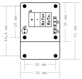
Figure 5 – Board with Electronics Drawing
