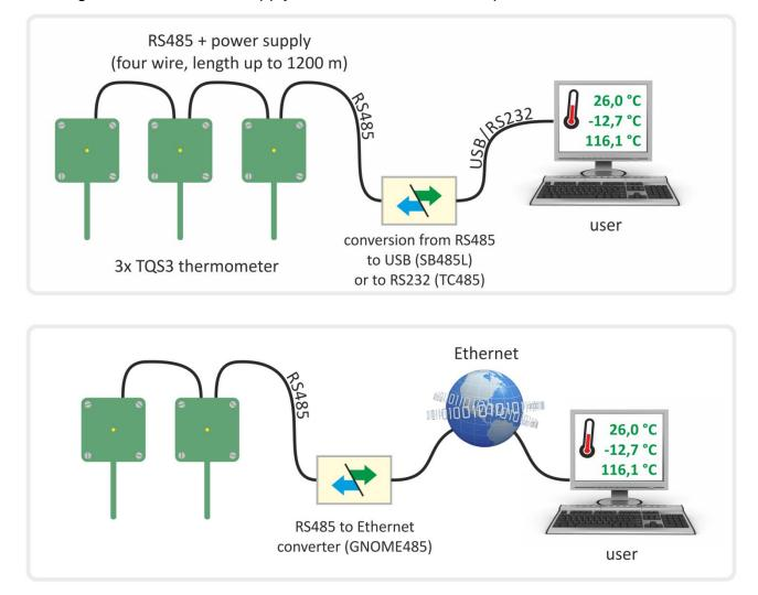
The module measures temperature using an integrated unit with the accuracy of  $\pm 0.5^{\circ}$ C. The TQS3 module contains an indicator which blinks to signalize the ongoing temperature measurement.
