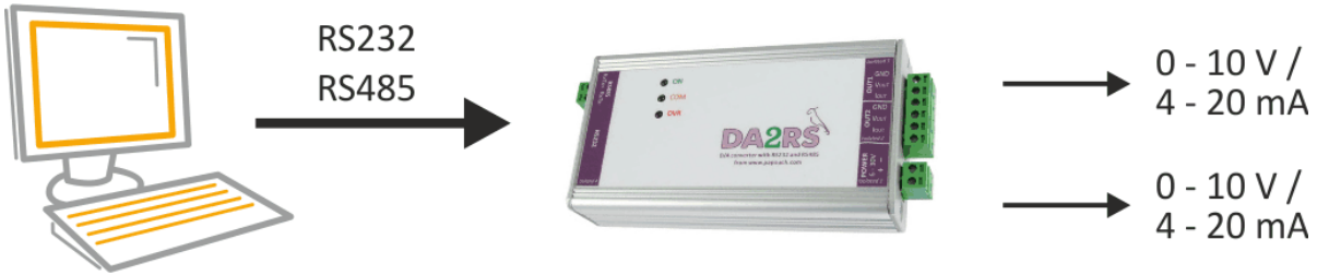
fig. 1 - Device function principle
